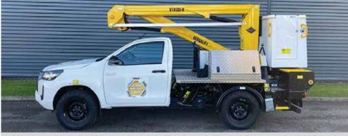
Manufactured from ultra-high strength steel, the Versalift profiled boom delivers exceptional rigidity and smooth operation on this low travel height platform.
