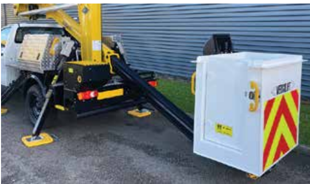
Safe access to bucket when in dock or from ground
