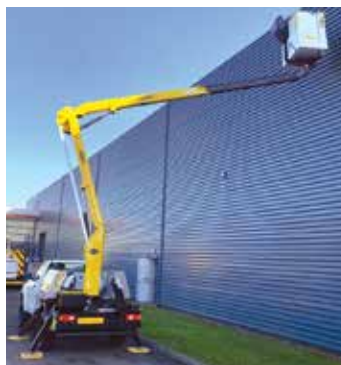
Zero tail swing on knuckle
