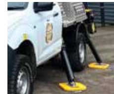
Double A-frame outriggers front and rear for compact setup
