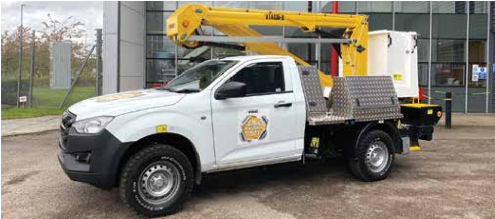
Manufactured from ultra-high strength steel, the Versalift profiled boom delivers exceptional rigidity and smooth operation on this low travel height platform.
