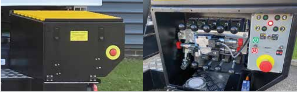
Hydraulic 12V DC emergency ground controls and emergency hand pump all located within a separate compartment to maximise bed space
